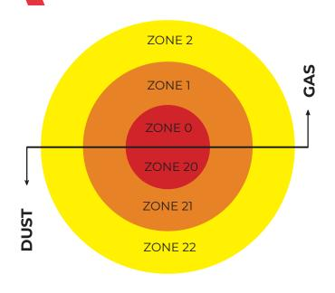
EXTRA-N-LED-2/21 is certified for ZONE 2 (explosive atmosphere of gases) and ZONE 21 (explosive atmosphere of dusts).
